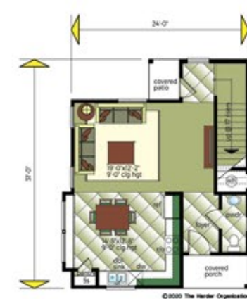
first floor plan plan: 1216
